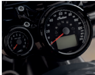
Among the many accessories available, there's a secondary rev counter with a gear change indicator that fits next to the original speedometer.
